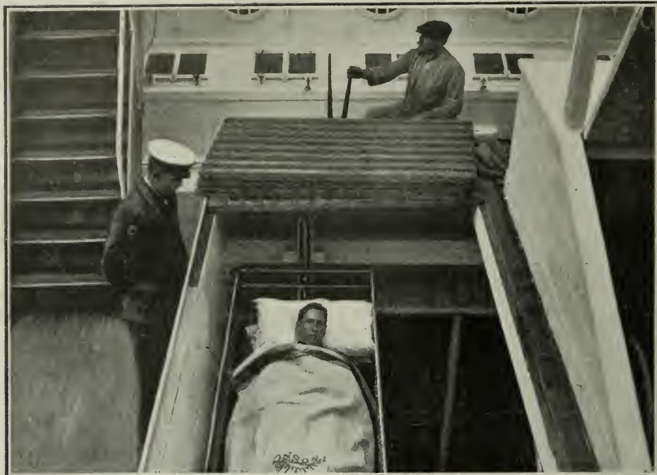
ON BOARD A HOSPITAL SHIP. Method of lowering a man into the wards.
